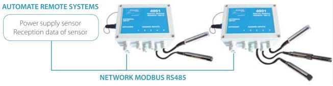
The module 4001 is compatible with all the sensors Modbus RS485 from PONSEL according to the following offer: sensor OPTOD (dissolved oxygen/Temperature), NTU (Turbidity Nephelometric), C4E (conductivity/salinity), pHEHT (pH, Redox, Temperature). The bus RS485 must be linear and is guaranteed functional on a maximal distance of 1km with a cable in pair twisted armored (type AWG26 for example).
