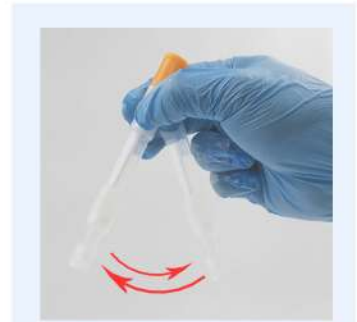
4. Shake to mix. Remove cap of the tip. Proceed to analysis using CompactDry™ of target parameter.
