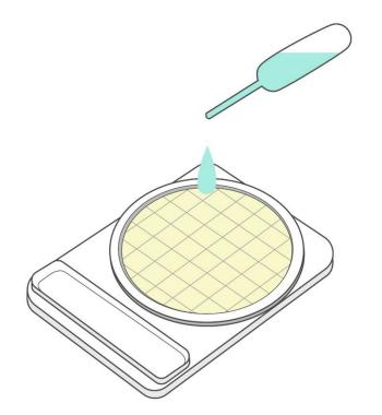
Pipette 1ml of homogenized specimen (to be further diluted if necessary) in the middle of dry sheet of Compact Dry CF.
