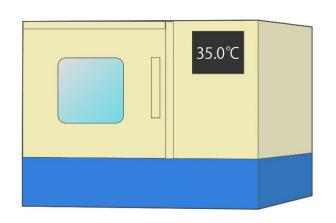
put in an incubator. Incubate 24 hours for CF at 35 +/- 2°C.
