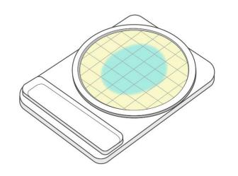
Specimen diffuses automatically and evenly into all over the sheet (total medium of 20 cm2) to transform it into gel within seconds.
