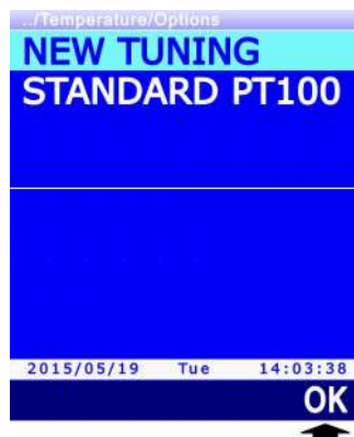
Fig. 13.3.2: types of calibration for the temperature sensor
