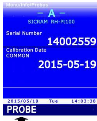
Fig. 11.2: information concerning the connected probes
