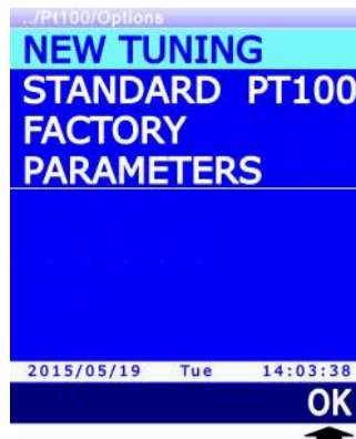
Fig. 13.1.1: PRT probe calibration types
