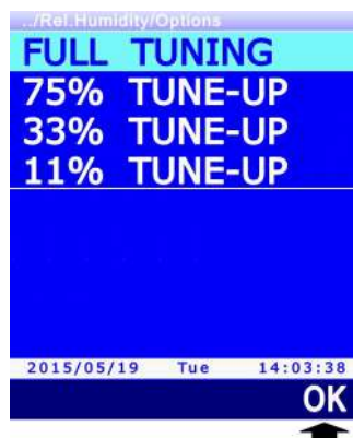
Fig. 13.3.4: types of RH sensor calibration
