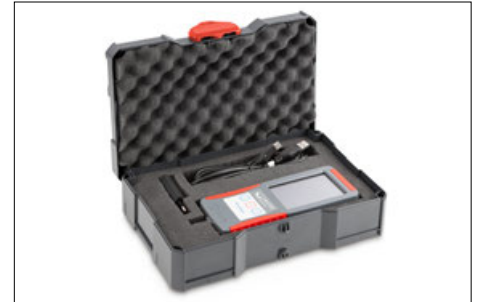
Supplied in a high-quality and robust system case (systainer® T-LOC) including mains adapter and USB cable type C
