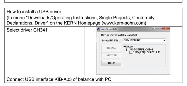
Go to device manager of PC and search for "USB Serial CH340 (COM6). (This COM Port will later be entered in Balance Connection.)
