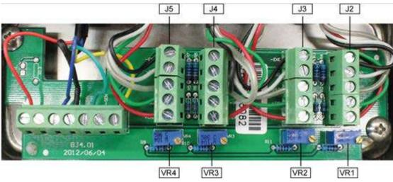
Adjustment of weighing cell 3 takes place at the potentiometer VR1.
