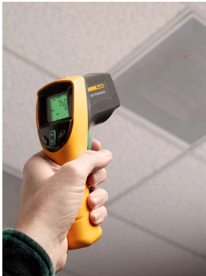
Measuring diffuser temperature.
