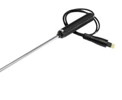
Protimeter 30cm HygroProbe BLD8755 is used to measure Relative Humidity (RH) and temperature in remote places such as HVAC ducts in HVAC applications or deep into a wall or floor cavity. This probe is used with Protimeter devices with an attached cable interface.
