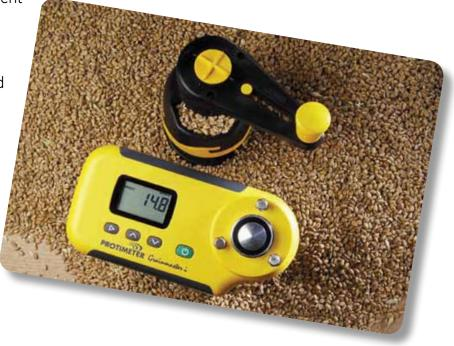
The Grainmaster is supplied in a pouch with grindercompressor unit, grain cup, sample spoon, brush and 'Quickcheck'. In addition to the 0-100 relative scale, 15 crop calibrations are pre-programmed into the instrument as listed below:
