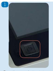
Press the power button to turn on the instrument.
