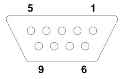
Pin 2: Transmit data Pin 3: Receive data Pin 5: Signal ground
