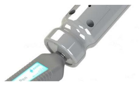
The calibrator should be the correct level for the configuration of the NoisePen, typically 94 or 114dB. Switch the calibrator on and press '**Calibrate**' in AnalyzerPlus. The result of the calibration will be reported, along with the present offset from the last factory calibration.
