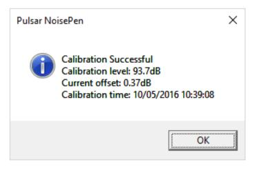
Only a Pulsar Instruments calibrator should be used with the NoisePen, as these have the appropriate correction factor for the difference between the free field and pressure responses of the microphone.
