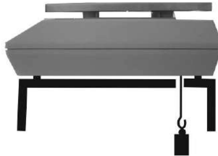
Fig. 1: Setup of balance for underfloor weighing
