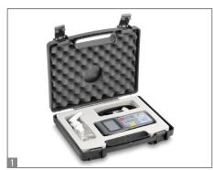
Hand-held measuring device for ultrasonic material thickness testing in Echo-Echo principle
