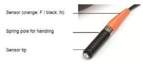
It is recommendable to effect several test measurements before the first use of the instrument. This way, further measurement errors can be avoided.
