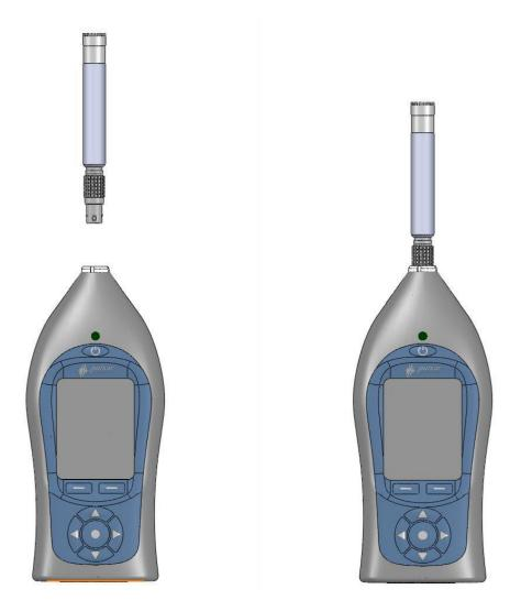
When connecting the preamplifier, please take care to align the locking tab (and red markings) on the preamplifier and instrument socket. Push the preamplifier connector into the instrument socket to connect them.
