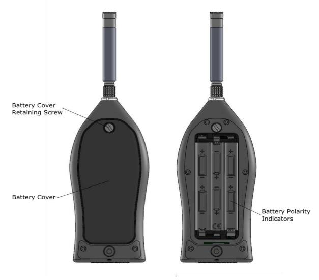
Please look carefully at the diagram inside the battery compartment that shows the correct polarity. After inserting the batteries in the correct orientation, replace the cover and tighten the battery cover retaining screw.
