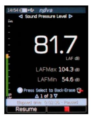
If your instrument has the Pause/Back Erase feature the measurement can be paused by pressing the Pause/Stop soft key.
