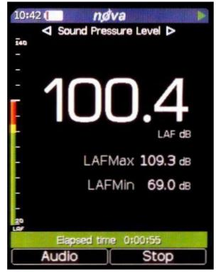
This view shows the Sound Pressure Level or SPL, with the maximum and minimum sound level (Lmax and Lmin) with a choice of A, C and Z frequency weightings.
