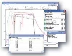
In addition to the monitor view, PicoLog can also display a graph, a spreadsheet and user notes. It can display them all at once, as shown here, or individually in any combination.
