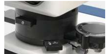
Bertrand lens, \lambda Slip, 360° rotatable analyser (removable)
