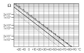
Since the resistance of the pH electrode is in the range of  $50-200~\text{M}\Omega$ , the current across the membrane is in the pico Ampere range. Large currents can disturb the calibration of the electrode for many hours.
